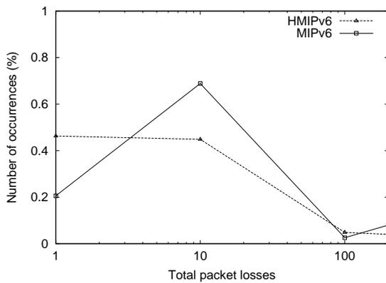
Figure 9. Histogram of the total packet losses considering random movement
