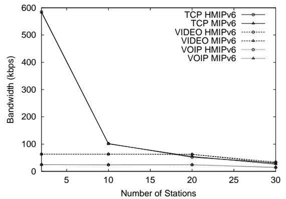
Figure 10. Impact of traffic sources on bandwidth
