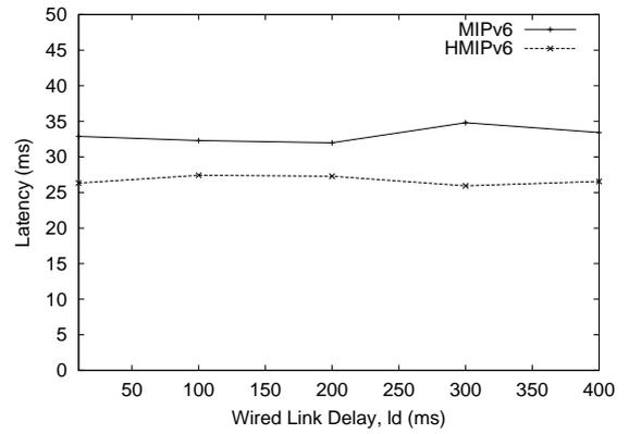
Figure 8. Impact of previous access router forwarding on handoff latency
