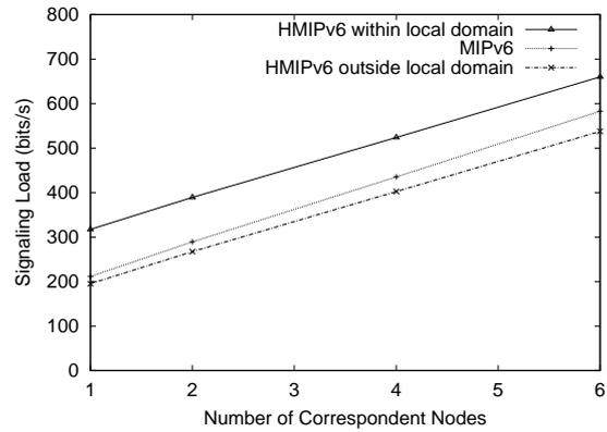
Figure 6. Impact of number of correspondent nodes on signaling load
