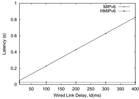
Figure 7. Impact of wired link delay on handoff latency
