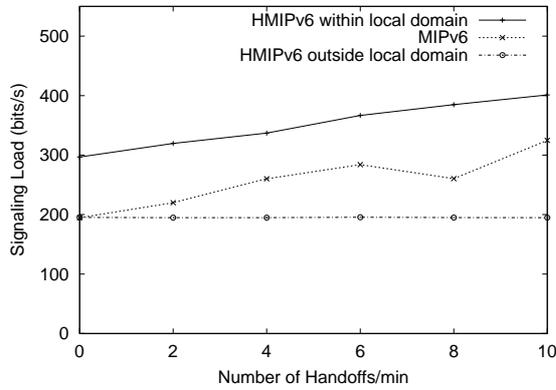
Figure 5. Impact of handoff rate on signaling load
